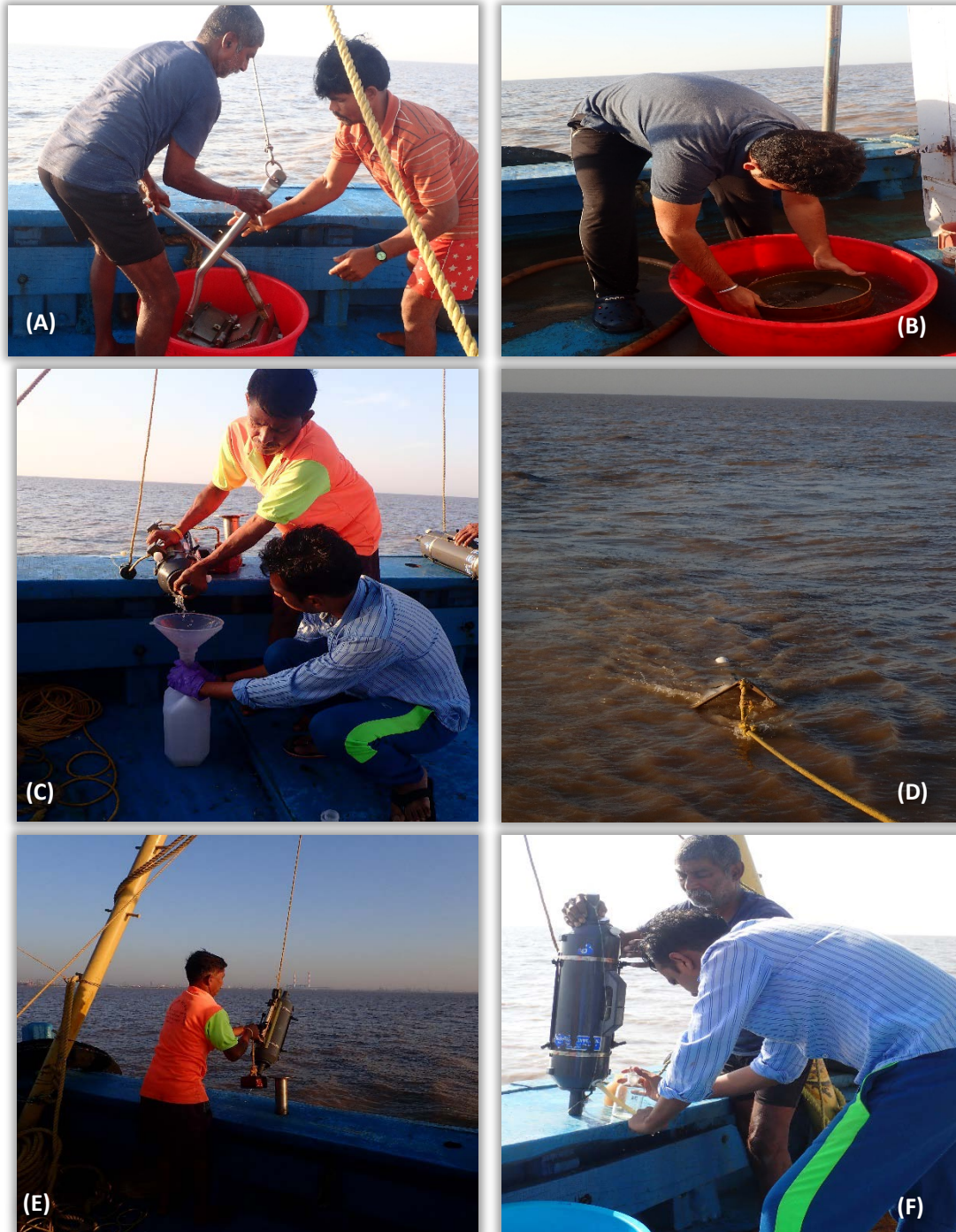
Plate 1: Photographs representing subtidal sampling at Dahej in October, 2022. A) Sediment collection using Van veen grab; B) Sieving of benthos sample; C) Collection of bottom water sample using Niskin sampler; D) Zooplankton sample collection using a Heron Tranter net; E) and F) Niskin sampler operation onboard for water sample collection.
