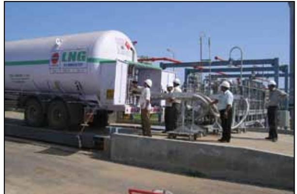
*Supply of LNG through Cryogenic Vehicles*
